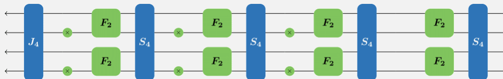
Streaming reuse with a streaming width of 2^k = 4
