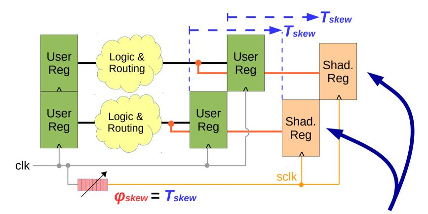
By placing and routing these shadow registers carefully, target *consistent* skew
